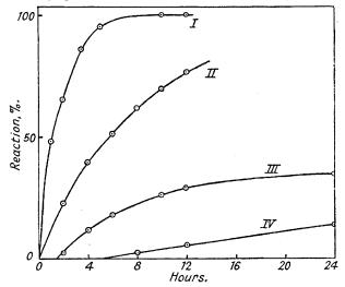
I, Liberation of bromide ion by 2n-NaOH. II, Liberation of bromide ion by n-NaOH. III, Formation of heto-acid by 2n-NaOH. IV, Formation of heto-acid by n-NaOH. (Slight losses of the 2: 4-dinitrophenylhydrazone, owing to its appreciable solubility in water, account for the displacement of curves III and IV from the origin.)
