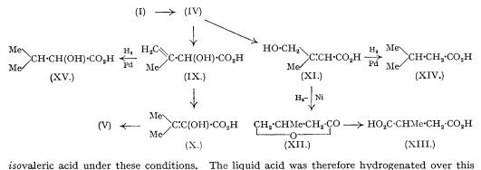
isovaleric acid under these conditions. The liquid acid was therefore hydrogenated over this catalyst and gave a mixture of  $\alpha$ -hydroxyisovaleric (XV) and isovaleric acid; the latter distilled with the water on evaporation of the solution, and a solid residue of the hydroxy-acid was obtained, thus confirming the structure of (IX).
